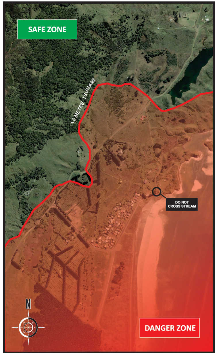
Mahanga 10m tsunami model ... an example of the models being used by Wairoa District Council to develop evacuation plans for coastal settlements.
